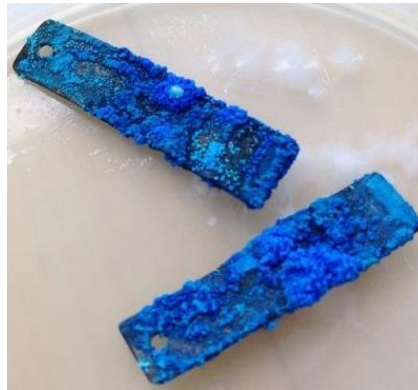
Fig. 3. Ammonia effects over copper [5]
